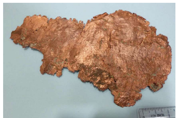
Figure 7.18 | Copper, which can be hammered into thin sheets, is malleable.
