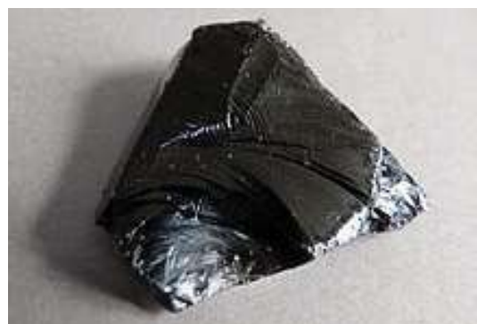
Figure 7.12 | This piece of igneous rock called obsidian has been hit with a hammer and is displaying conchoidal fracture.
